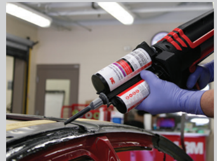
May be used for bonding door skins, quarter panels, roof skins, box sides, van/utility vehicle sides and rocker panels when recommended by OEMs.
