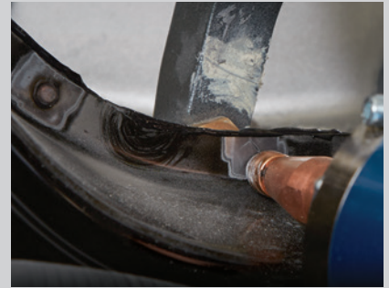
3M™ Panel Bonding Adhesive can be welded through within working time using squeeze-type resistance spot welding to form a weld bonded joint.
