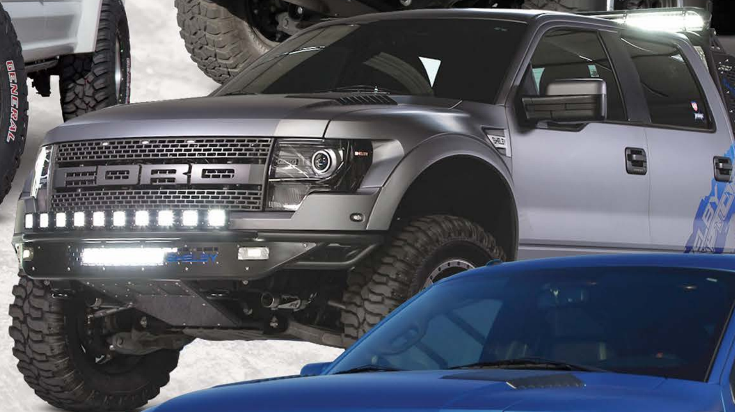
10 - 14 FORD RAPTOR RACE SERIES™ R FRONT BUMPER With Aluminum Valence Option & 10 Cube Light Mounts Option F014532910103
