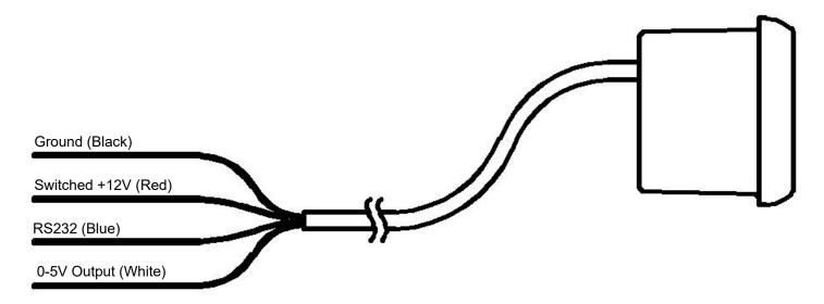
Figure 1. Connection Diagram
