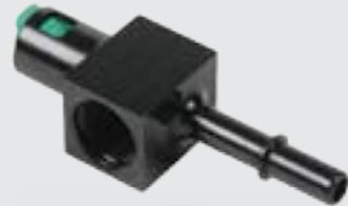
3/8" Quick Connect with AN-08 fuel access port and 1/8" NPT gauge port : #15121
