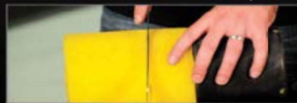
Cut hanger 1 in SHORTER than tank depth
