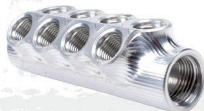
P/N 14602 10 Port Fuel Distribution Log (2) ORB-10, (8) ORB-06
