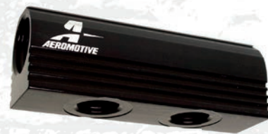
P/N 14601 4 Port Fuel Distribution Log (2) ORB-08, (2) ORB-06
