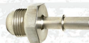
P/N 15104 3/8" Male Quick Connect / AN-10 Male (GM LT-1 filter inlet)
