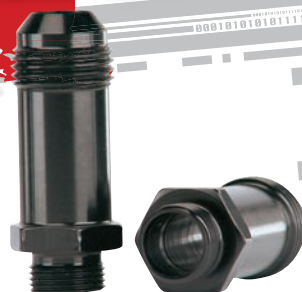
P/N 15208 Demon Carb AN-08 to 9/16" x 24 Thread Float Bowl Fitting
