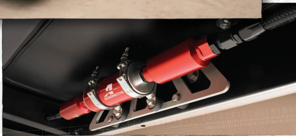
Murray Pfaff's Imperial Speedster Built and Designed by: Pfaff Designs Fueled by: Aeromotive A750 Fuel Pump (P/N 11106)
