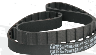
21110 Timing Belt - 1/2" wide Neoprene w/ fiberglass cord, 60 groove (22.5"), L pitch (.375")
