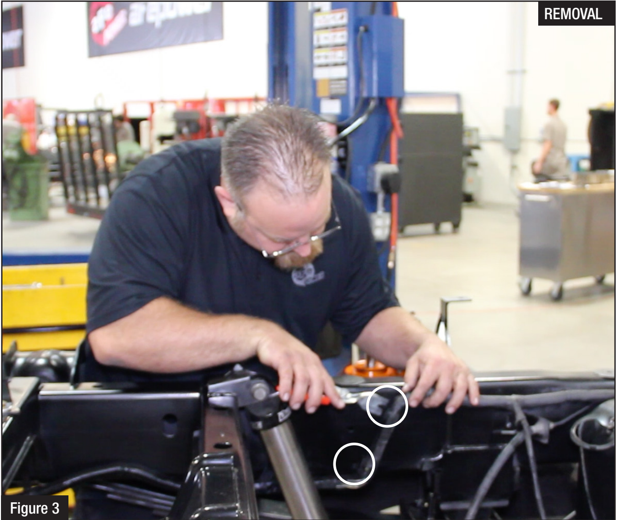
Step 3: Remove the factory wire harness from the two mounting holes. (As circled above)
