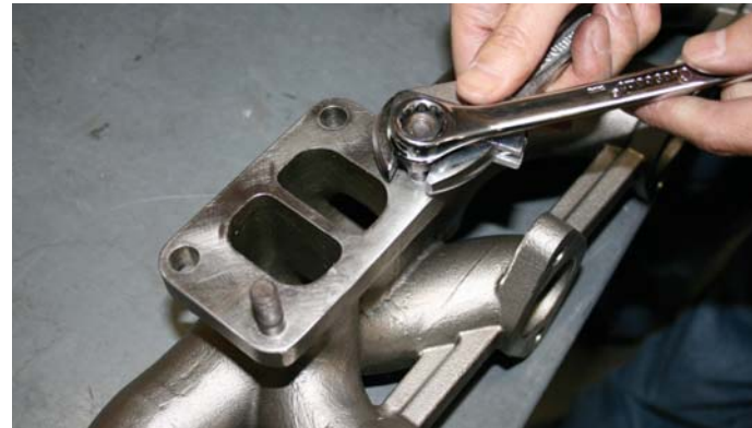
8 – Install studs provided on aFe manifold. Use 2 M10x1.5 nuts and turn them into each other so that they no longer spin freely. Next turn the top nut only to tighten the stud. Remove nuts from stud.
