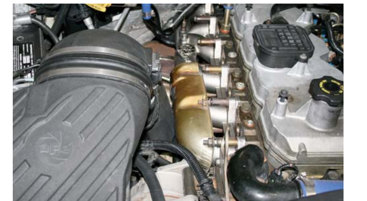
15 – Re-install heat shield and air intake turbo inlet. Reconnect the negative (-) battery terminals. Your installation is complete. Thank you for choosing aFepower!
