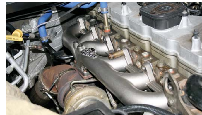
11 – Install aFe exhaust manifold. IMPORTANT: Use new exhaust manifold gaskets available from your local Dodge dealer. Manifold gaskets part number 513589AA and turbo flange gasket part number 3949530.
