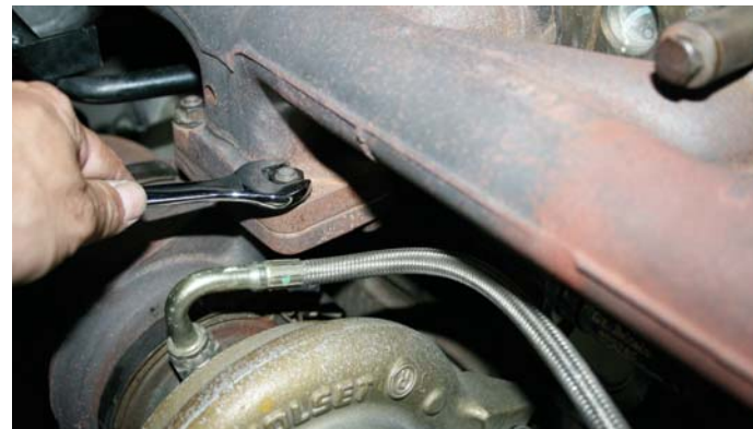
5 – Remove 4 nuts holding the turbo to the stock manifold. The 2 back nuts are reached from underneath the truck. NOTE: No need to remove the turbo or loosen the exhaust. Wear safety glasses.
