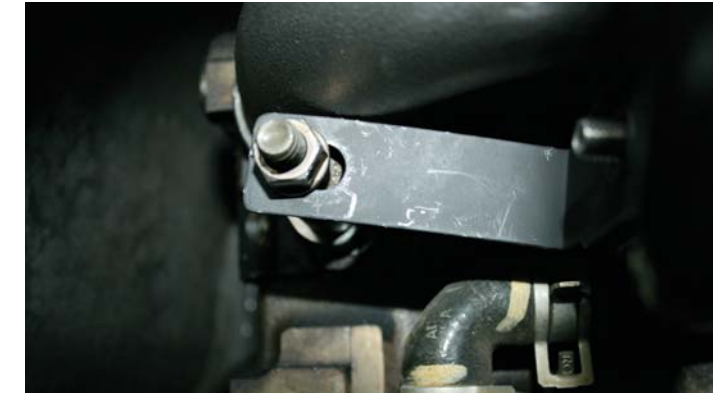
13 – If using bracket provided, install on bolt farthest to the back of the manifold after bolts are tightened.
