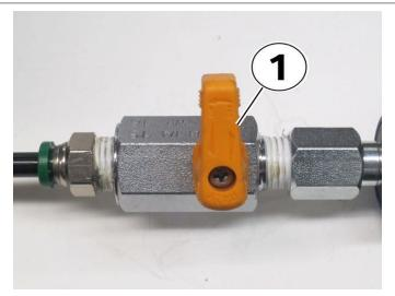
Step 9: The air supply valve (1) is still off.
