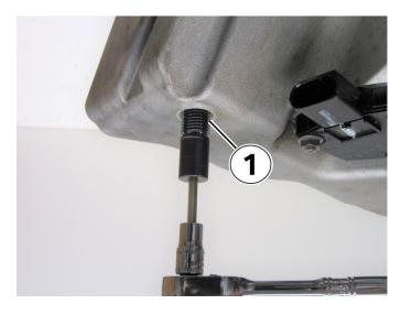
**Step 20:** Inset the alignment pin (1) with a 1/8 or 5mm Allen socket until it is flush with the oil pan surface.
