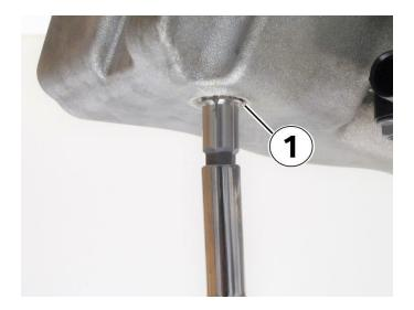
**Step 17:** Continue turning the tap until the last thread is flush with the outer pan surface (1).
