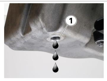
**Step 6:** Engine oil will begin to exit the oil pan again (1) with the air supply valve in the on position.
