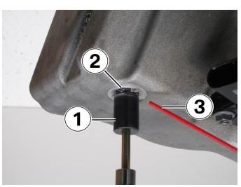
**Step 21:** Install the re-facing tool into a drill (1). Recommended drill setting is:
