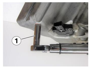
**Step 26:** Torque the drain plug (1).
