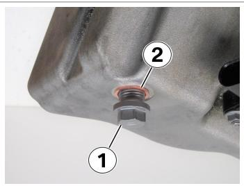
**Step 24:** Install the new drain plug that is supplied in this repair kit.
