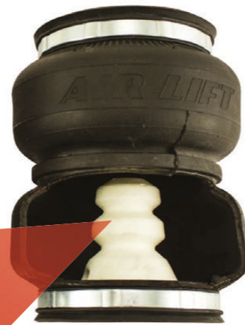
Cutaway of air spring showing internal jounce bumper.
