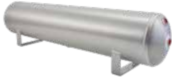
Aluminum 4 Gallon P/N 11955 - Raw Finish P/N 12955 - Polished (2) 1/4" NPT End Ports (2) 3/8" NPT End Ports (1) 1/4" NPT Drain Port Dimensions: 30"L X 6"D
