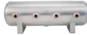
Aluminum 2 1/2 Gallon P/N 11958 - Raw Finish P/N 12958 - Polished (4) 1/4" NPT Face Ports (1) 1/4" NPT Drain Port Dimensions: 20"L X 6"D
