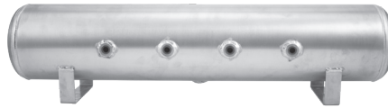
Aluminum 4 Gallon P/N 11957 - Raw Finish P/N 12957 - Polished (4) 1/4" NPT Face Ports (2) 3/8" NPT End Ports (1) 1/4" NPT Drain Port Dimensions: 30"L X 6"D
