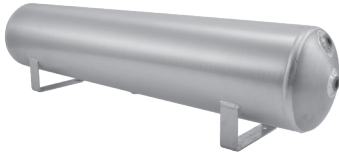
Aluminum 4 Gallon P/N 11955 - Raw Finish P/N 12955 - Polished (2) 1/4" NPT End Ports (2) 3/8" NPT End Ports (1) 1/4" NPT Drain Port Dimensions: 30"L X 6"D
