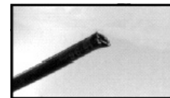
Bad cut - flattened
