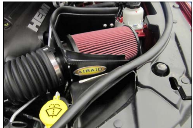
17. Install the Airaid Premium Filter.
