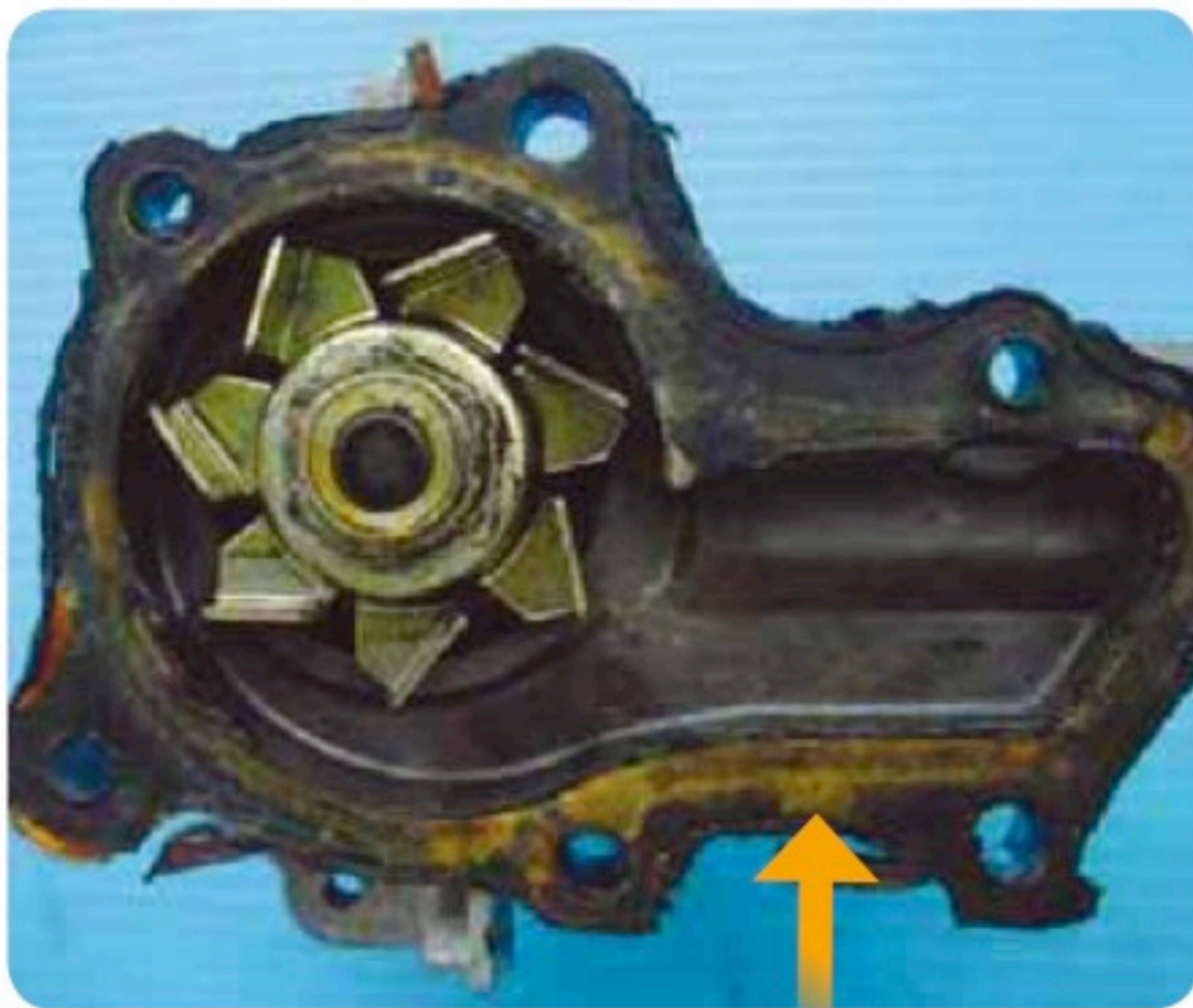
Insufficient accuracy on the mounting surface.
