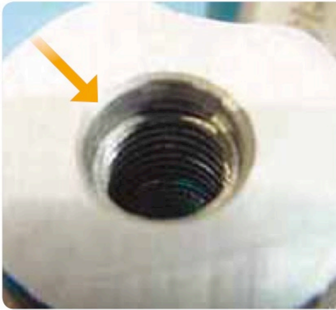
Threads have been stripped.
