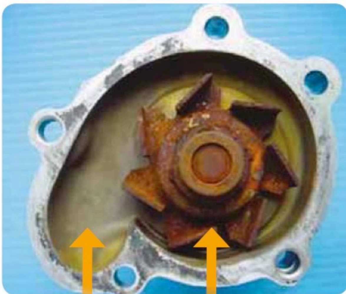
Contamination of water pump body
