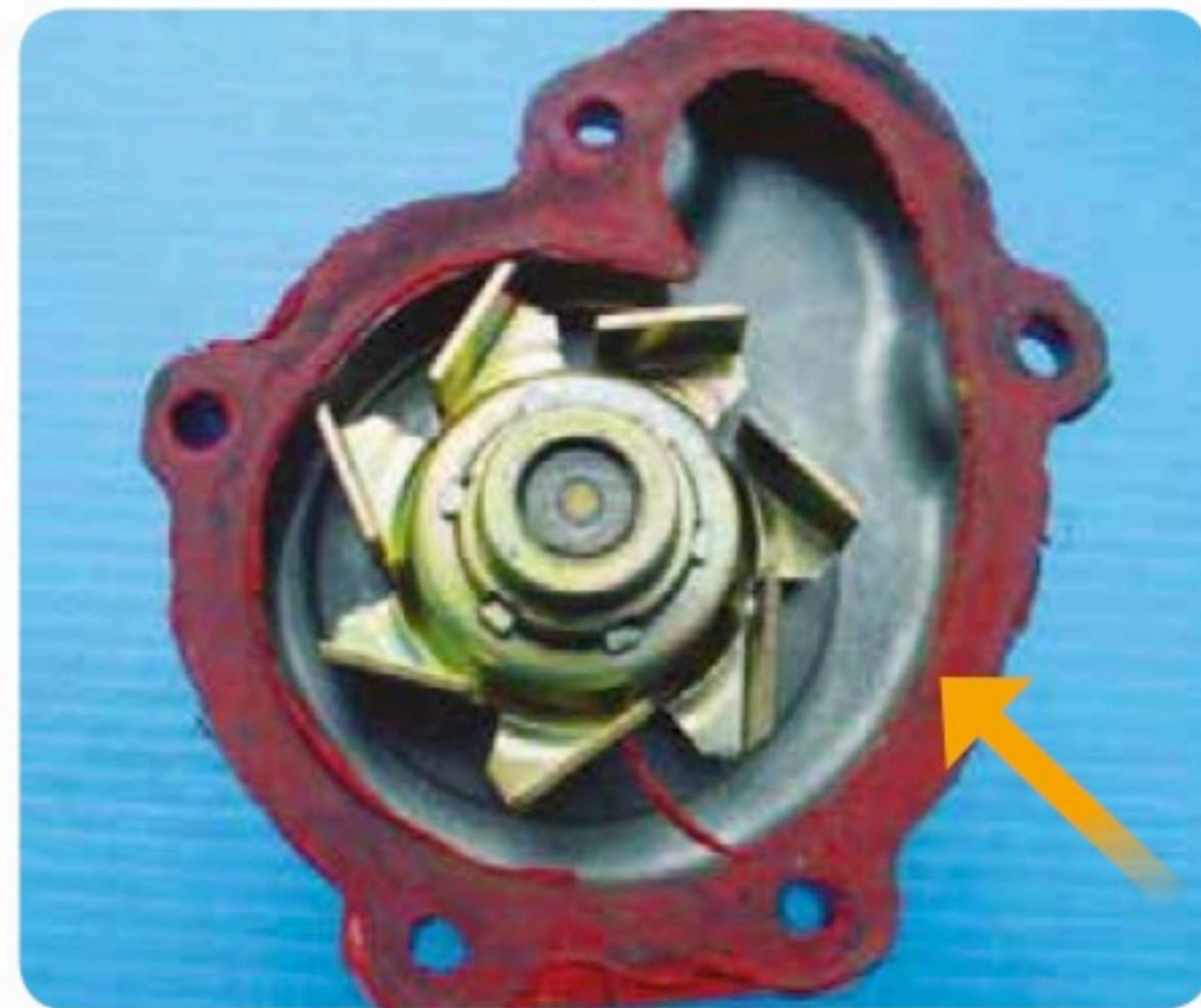
Gasket performance has degraded.
