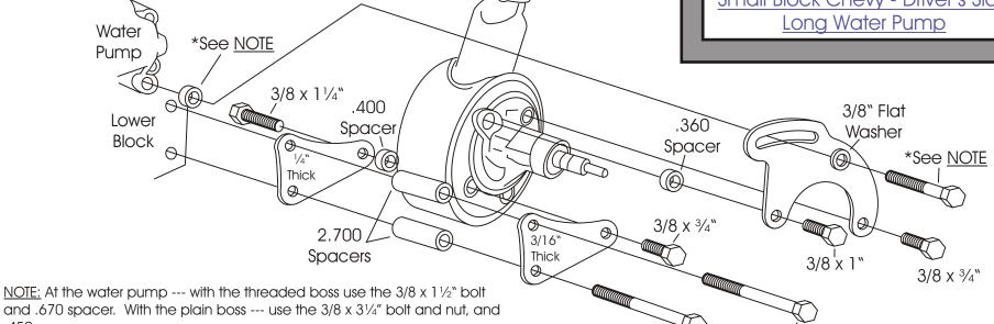
If your pump has a stud at the lower rear pivot point, remove it and use the 11/4" bolt and .400 spacer.
