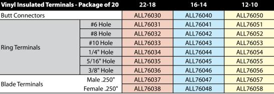
Vinyl-insulated terminals are the most popular crimp terminal used in a variety of applications. PVC insulated sleeve is securely attached to terminal and has a flared end for easy installation.
