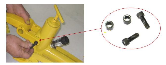
9. Replace the pivot pin and install the e-clips on both sides using a hammer.
