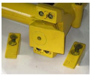
5. Using a steel punch, knock out the roll pin and remove the center foot. Once the pin is remove, gently tap the foot to remove.
