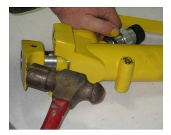
6. Install the new center foot and drive the roll pin in place with a punch and a hammer.
