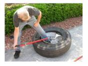
4. Keeping tool engaged, pull handle back to starting side. Be sure handle returns almost to the ground. ( See next two pictures)
