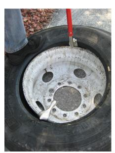
3. Place bead keeper on the wheel to hold the bead as the tire is mounted. Begin working around the edge where the bead is not yet mounted.
