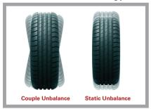
A unique balancing system (unbalance correction methodology) that minimizes both static and couple unbalance
