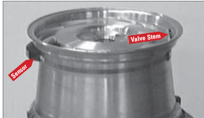
Figure 31 - Wheel with Low Pressure Sensor/Transmitter
