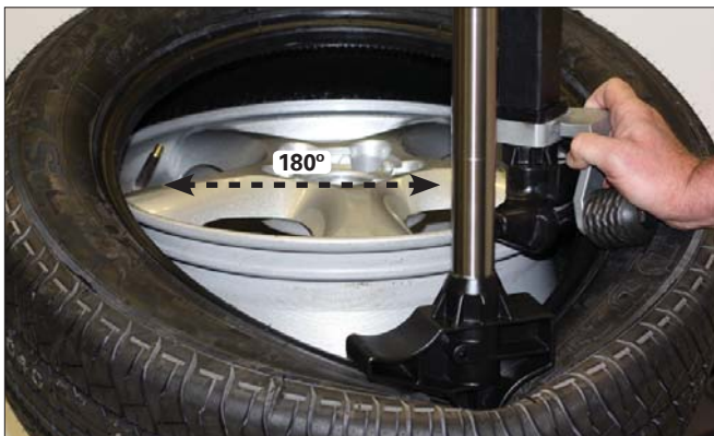
Figure 21 - Position Valve Stem 180° Ahead of Mount Tool
