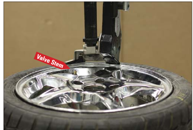
Figure 50 - Position Valve Stem Behind Leverless Demount Tool
