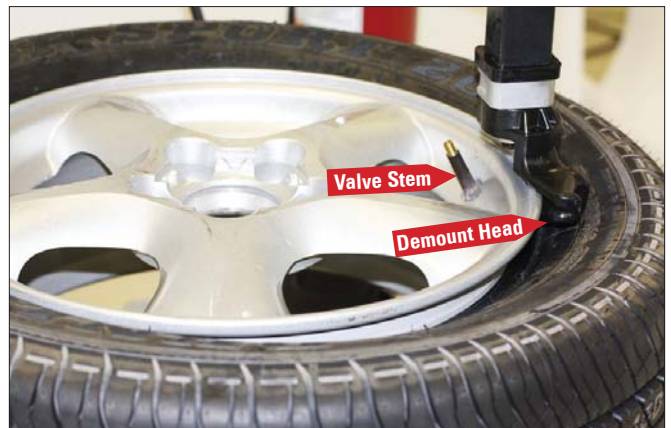
Figure 36 - Position Valve Stem Under Demount Tool
