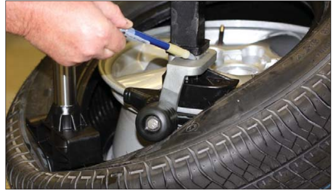
Figure 22 - Duckhead Roller Properly Mounted On Bracket
