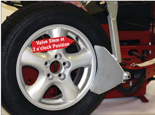
Figure 3 - Position Tire and Bead Loosener Shoe with Valve Stem in 2 o'clock Position.
