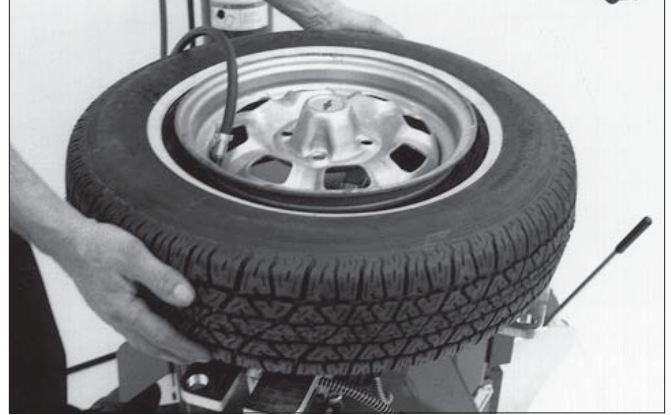
Figure 25 - Lift Tire Upwards for Bead Sealing
