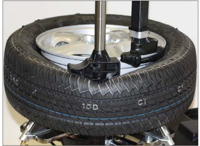
Figure 34 - Helper Foot Depressing Sidewall of Tire
