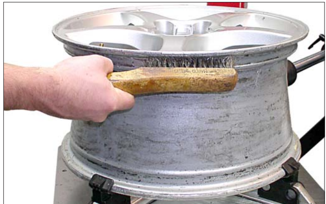
Figure 19 - Inspect and Clean the Wheel
