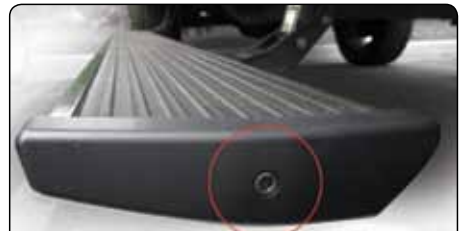
NEW STYLE STEP EXTRUSION Trim strip compatible only with new Style step extrusion identified by the single-bolt end cap shown.
