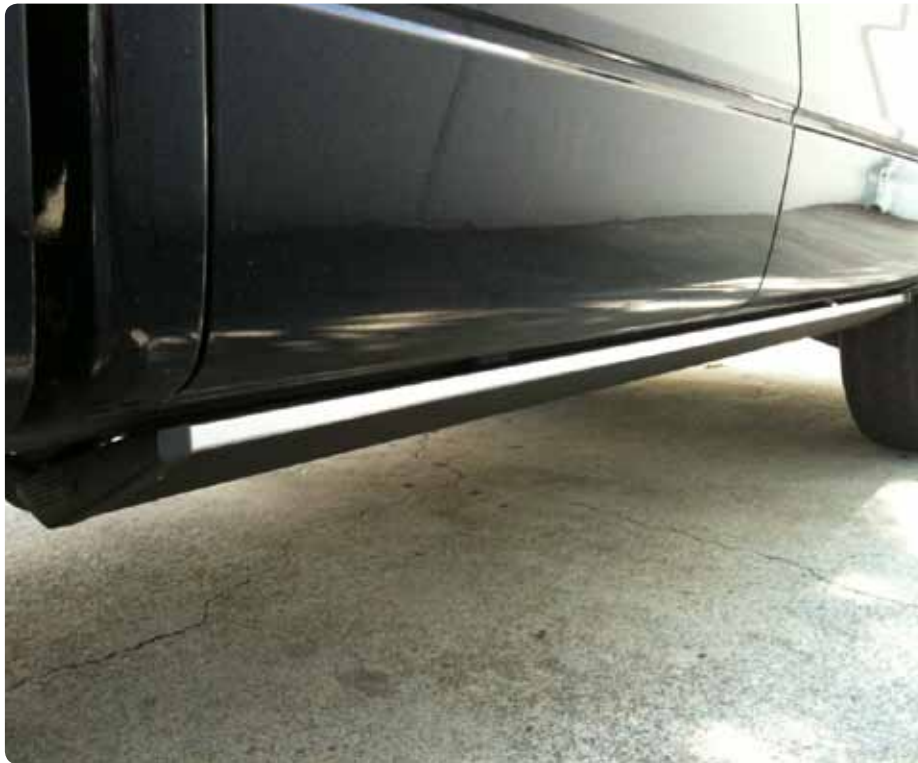
75149-01A Stainless-Steel Trim Strip - 79" (Set of 2) Requires new style step extrusion.
