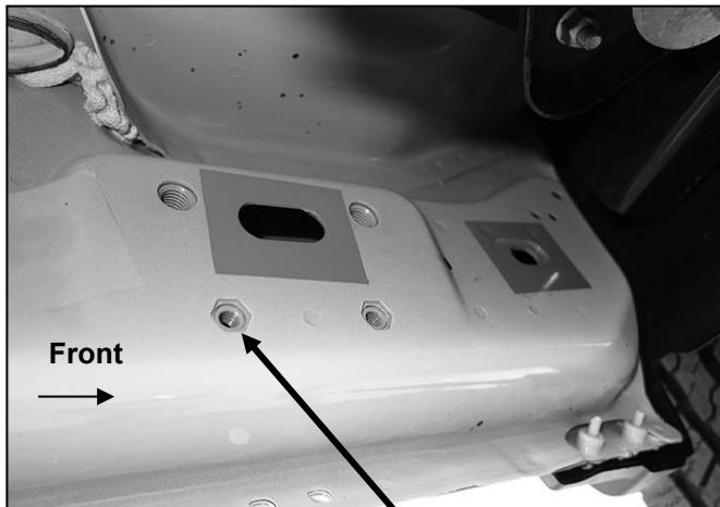
(Fig 7) Driver side front mid 2015-on, an example of models with factory installed threaded inserts
