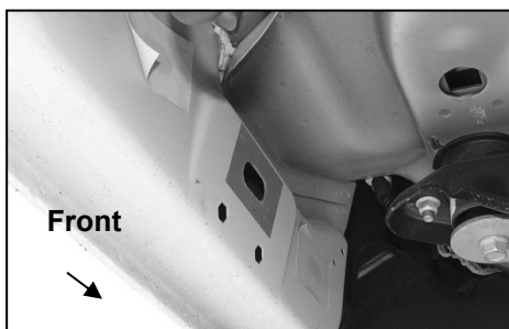
(Fig 1) 2009-mid 2015 Driver/Left front mounting location (No factory holes in pinch weld 2009-2011 models)
