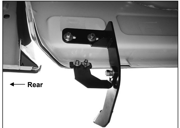
(Fig 16) Driver/Left rear Mounting Bracket assembly
