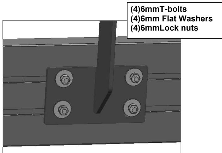
Fig 16 Bracket Installation
