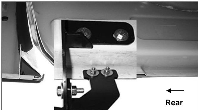
(Fig 16) Driver/Left rear upper Mounting Bracket assembly
