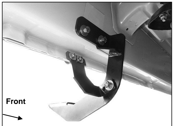
(Fig 14) Attach Driver/Left Support Bracket to back of Center Mounting Bracket
