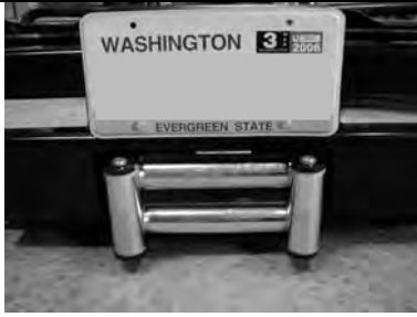
Fitting with winch, number plate above RFL
