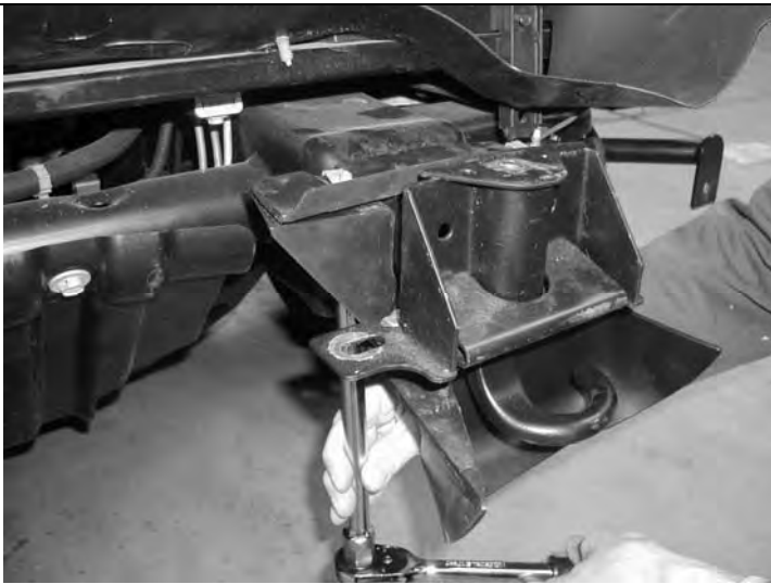
1.5 Remove plastic shrouds around chassis
