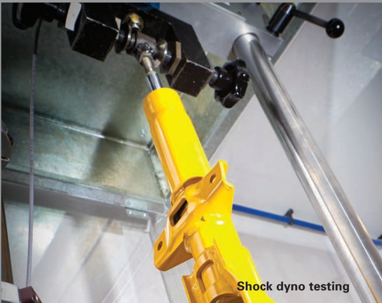
Vehicle specific shock valving analysis
