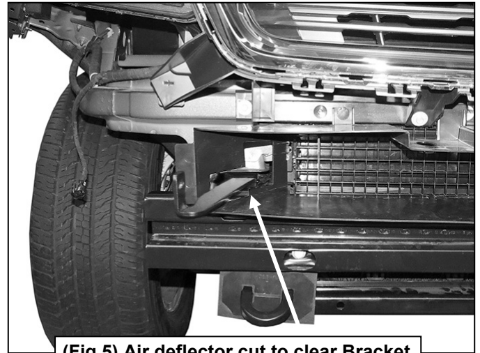
(Fig 5) Air deflector cut to clear Bracket
