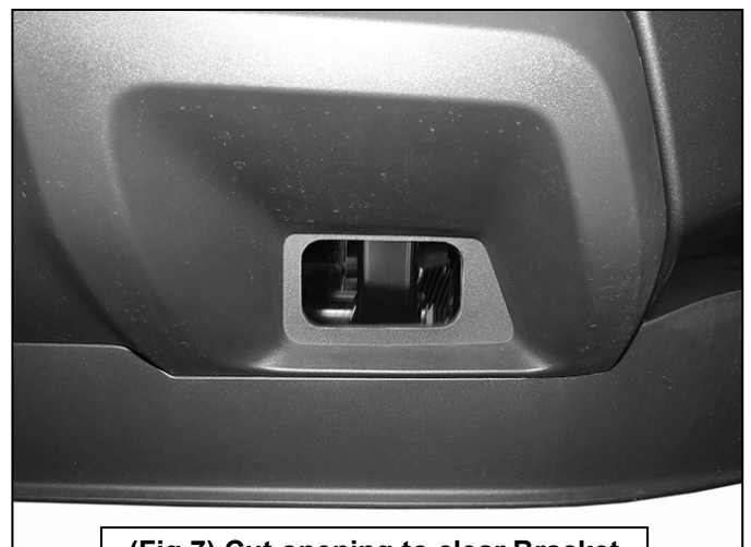
(Fig 7) Cut opening to clear Bracket
