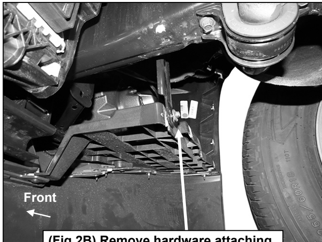
(Fig 2B) Remove hardware attaching plastic fill panel to inner fender
