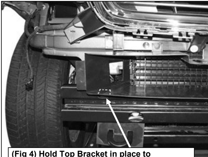
(Fig 4) Hold Top Bracket in place to determine area to cut from air deflector
