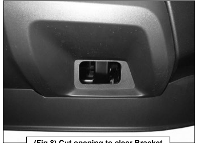
(Fig 8) Cut opening to clear Bracket
