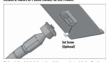
Optional: Attach included metal conduit to console to minimize vibration.
