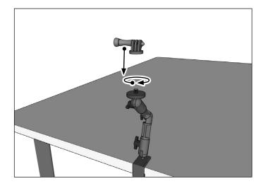
3 Unscrew lateral screw and insert GoPro HERO (sold separately) to the adapter. Re-insert lateral screw.
