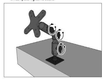
2 Attach the pedestal to the mounting surface through the AMPS base plate. Choose the screws that will work best on the chosen mounting surface. Use anchors if necessary.
