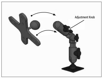
3 Loosen adjustment knob to adjust angle of pedestal and position of VESA plate. Tighten to secure.
