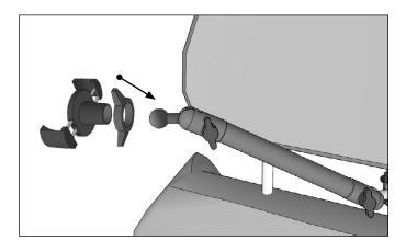
2 Loosen the adjustment knob on the pedestal, remove the drill base, and position the pedestal over the mount's ball. Retighten knob and set pedestal to desired angle.
