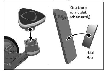
Place metal plate on the smartphone in contact with the magnet head on the pedestal to attach. Rotate or adjust angle as needed.
