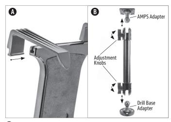
Attach the mount arm to the round drill base adapter. Attach the holder to the mount arm. Tighten adjustment knobs to secure.
