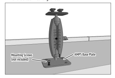
Insert smartphone or midsize tablet by placing it on the two lower legs and pushing down on the spring-loaded bottom of the holder. Loosen adjustment knob to adjust position & angle. Retighten to set.
