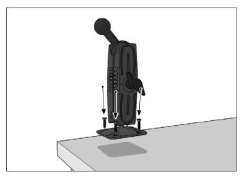
Place adjustment ring over the pedestal ball and snap the RoadVise Holder onto the pedestal.
