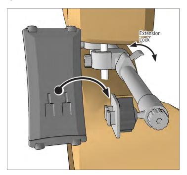
To mount a device, push down on legs and place in holder.
