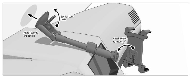
2 Adjust length of mount as necessary by unlocking extension arm. Lock arm when desired length reached. Insert device by pushing down on lower legs of spring-loaded holder.
