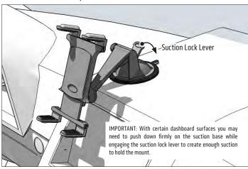
3 Insert tablet into holder by pushing down on the bottom spring-loaded support legs with the tablet. Slide the top of the tablet under the top support legs until it fits snuggly in the holder.
