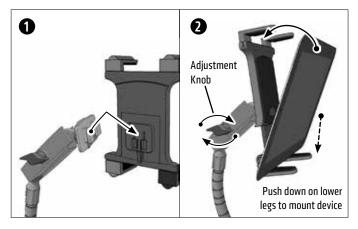
The Slim-Grip Universal Tablet Holder fits tablets with 7" - 18.4" screen size. It includes 4 short, 2 medium, and 4 long support legs. Select a combination of 4 support legs in conjunction for use with the spring-loaded holder to achieve the perfect fit for your tablet.
