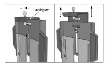
2 Unscrew the three screws/washers at the back/center of the holder to adjust the tablet holder's height to the tablet (not included). Retighten the screws/washers to secure.
