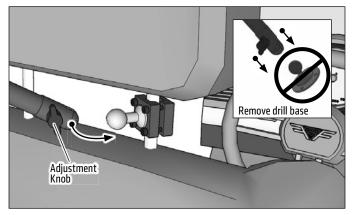
Insert tablet into holder by pushing down on the bottom springloaded support legs with the tablet. Slide the top of the tablet under the top support legs until it fits snuggly in the holder.
