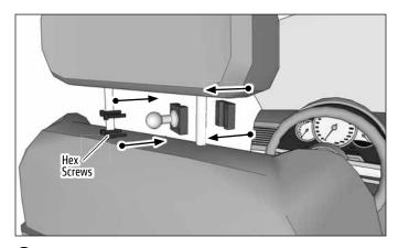
Attach the holder to the mount by inserting the Dual T-Tabs into the holder's Dual T-Slots and pushing down to lock. Loosen adjustment knob to set desired position of holder and retighten.
