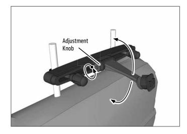
4 Insert tablet by placing it on the two lower legs and pushing down on the spring-loaded bottom of the holder. Loosen tightening ring to adjust rotation, position, or angle. Retighten to set.
