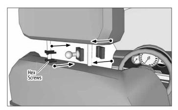
Attach the holder to the mount by inserting the Dual T-Tabs into the holder's Dual T-Slots and pushing down to lock. Loosen adjustment knob to set desired position of holder and retighten.
