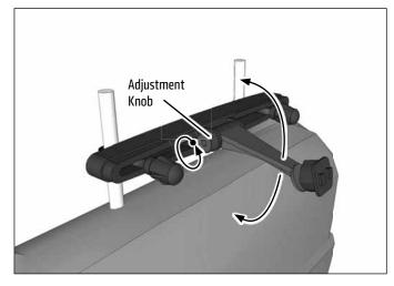
Place tablet on support legs, push down firmly on grip arm to hold tablet. Adjust the mount to desired position; release tablet by pushing the grip arm release. Loosen tightening ring to adjust rotation, position, or angle. Retighten to set.
