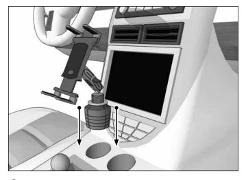
Insert tablet by pushing down on the lower legs to engage the spring-loaded mechanism. Adjust support legs as necessary.
