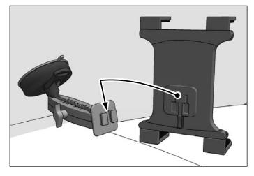
**OPTIONAL:** For dashboard mounting, use included adhesive disk. Clean surface before applying and let dashboard disk adhesive cure for 24 hours before use.
