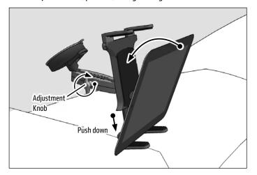
2 Attach Slim-Grip tablet holder by sliding the Dual T-Tabs on the pedestal head into the Dual T-Slots of the holder.
